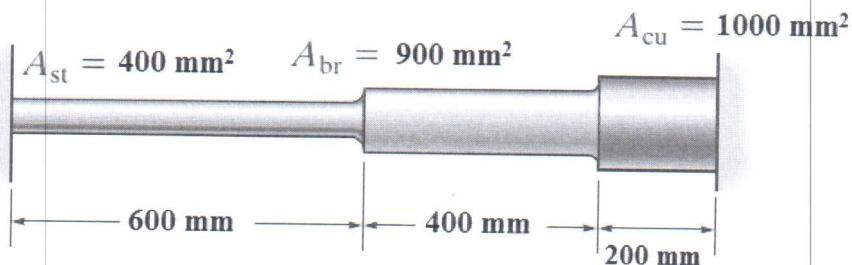
Three bars each made of different materials are connected together and placed between two walls when the temperature is  $T_1 = 12\text{°C}$ . Determine the force exerted on the (rigid) supports when the temperature becomes  $T_2 = 18\text{°C}$ . The material properties and cross-sectional area of each bar are given in the figure. ( Sketch the free body diagram.)
