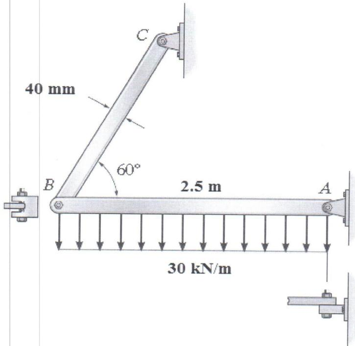
Determine the required thickness of member BC and the diameter of the pins at A and B if the allowable normal stress for member BC is  $\sigma_{allow}=200$  MPa and the allowable shear stress for the pins is  $\tau_{allow}=70$  MPa. ( Sketch the free body diagram for each member)
