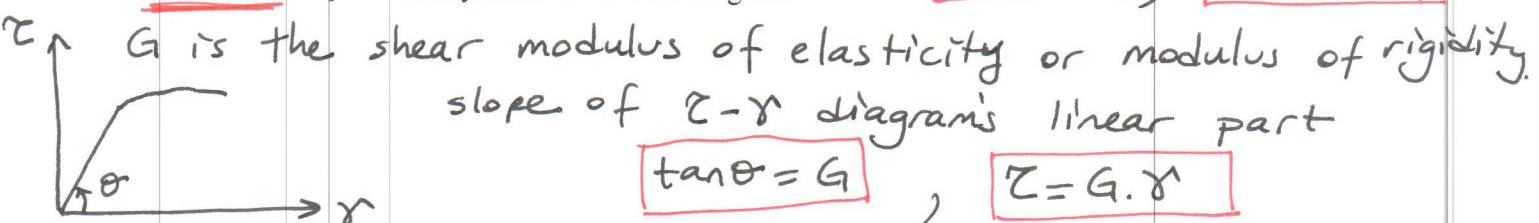
$G$  is the shear modulus of elasticity or modulus of rigidity
