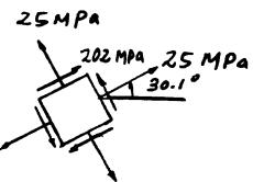
**9-87** The post has a square cross-sectional area. If it is fixed-supported at its base and the loadings are applied at its end as shown, determine (a) the maximum in-plane shear stress developed at A and (b) the principal stresses at A.
