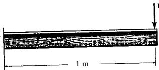
As shown on FBD,  $V_{\max} = 10 \text{ kN}$
