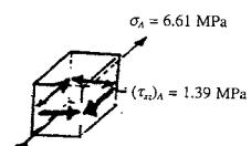
**8-57** The 1-mm-diameter rod is subjected to the loads shown. Determine the state of stress at point *B*, and show the results on a differential element located at this point.
