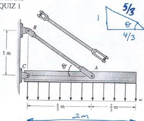
Determine the intensity  $w$  of the maximum distributed load that can be supported by the hanger assembly so that an allowable shear stress of  $\tau_{allow} = 100 \text{ MPa}$  is not exceeded in the 12-mm-diameter bolts at A and B, and an allowable tensile stress of  $\sigma_{allow} = 150 \text{ MPa}$  is not exceeded in the 15-mm-diameter rod AB.
