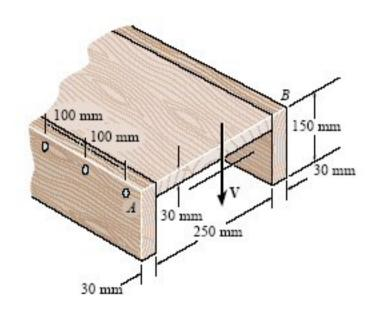
7-86. Determine the maximum shear stress acting at section a-a in the beam.
