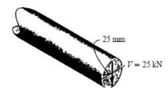
Determine the largest shear force V that the member can sustain if the allowance shear stress is  $\tau_{\text{allow}} = 8 \text{ MPa}$ .
