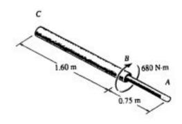
5-79. The shaft is made from a solid steel section AB and a tubular portion made of steel and having a brass core. If it is fixed to a rigid support at A, and a torque of  $T = 50 \text{ N} \cdot \text{m}$  is applied to it at C, determine the angle of twist that occurs at C and compute the maximum shear and maximum shear strain in the brass and steel.  $G_{st} = 80 \text{ GPa}$ ,  $G_{br} = 40 \text{ GPa}$ .
