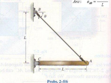
**2-10.** The wire AB is unstretched when  $\theta = 45^{\circ}$ . If a vertical load is applied to bar AC, which causes  $\theta = 47^{\circ}$ , determine the normal strain in the wire.
