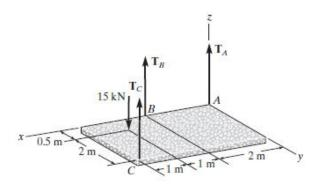
Equations of Equilibrium. Referring to the *FBD* of the slab shown in Fig. *a*, we notice that  $T_C$  can be obtained directly by writing the moment equation of equilibrium about the *x* axis.
