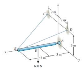
Force And Position Vectors. The coordinates of points A, B, C, D and E are A(0, 0, 0), B(6, 0, 0), C(0, -2, 3) m, D(0, 2, 3) m and E(3, 0, 0) m respectively.
