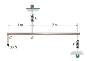
Equations of Equilibrium.  $\mathbf{F}_A$  and  $\mathbf{F}_B$  can be determined directly by writing the moment equation of equilibrium about points *B* and *A* respectively by referring to the *FBD* of the bar shown in Fig. *a*.
