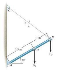
$$\zeta + \Sigma M_A = 0; \qquad -800(1.5\cos 30^\circ) - 350(2.5\cos 30^\circ) \\ + \frac{4}{5}F_{CB}(2.5\sin 30^\circ) + \frac{3}{5}F_{CB}(2.5\cos 30^\circ) = 0 \\ F_{CB} = 781.6 = 782 \text{ N} \\ \Rightarrow \Sigma F_x = 0; \qquad A_x - \frac{4}{5}(781.6) = 0 \\ A_x = 625 \text{ N} \\ + \uparrow \Sigma F_y = 0; \qquad A_y - 800 - 350 + \frac{3}{5}(781.6) = 0 \\ A_y = 681 \text{ N}$$
