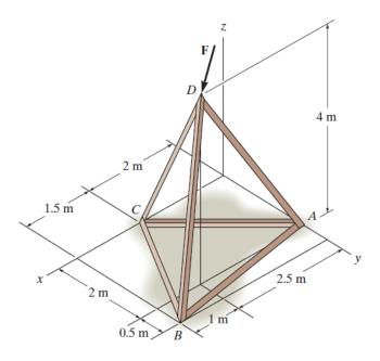
Determine the magnitude of the moment of the force F = {50i - 20j - 80k} N about the base line CA of the tripod.
