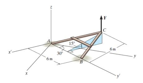
5. Determine the magnitude of the moment of each of the three forces about the axis AB. Solve the problem **a**) using a Cartesian vector approach and **b**) using a scalar approach.
